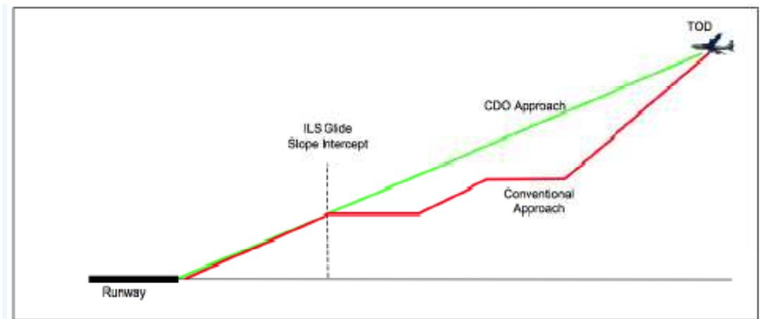
C4.3 The noise 'footprint' is reduced because the aircraft remains higher for longer and the engines remain at lower thrust (i.e. no need to spool up to level off). Due to the lower thrust settings, the CDO also results in reduced fuel burn and less green house gas emissions.
